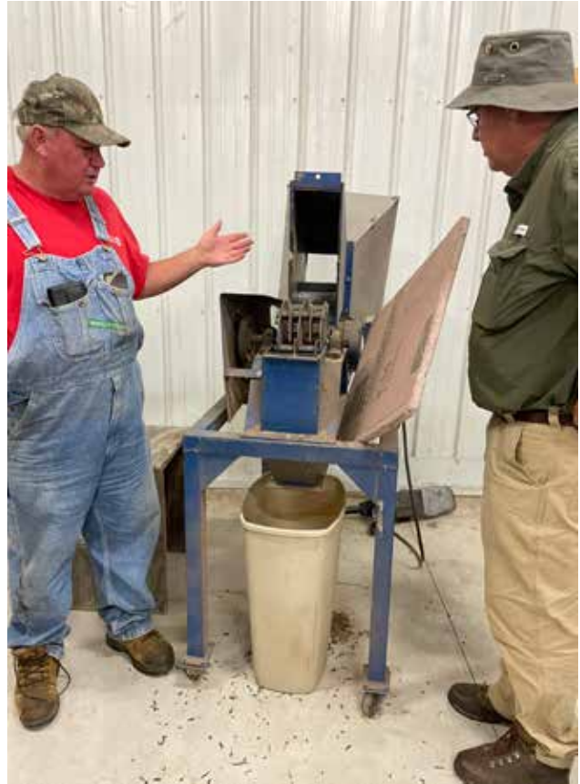
Above: Keith shows LHMMN Dave Gamet how the hammer mill is used at Dunn Ranch Prairie to process seed collected in the field.
